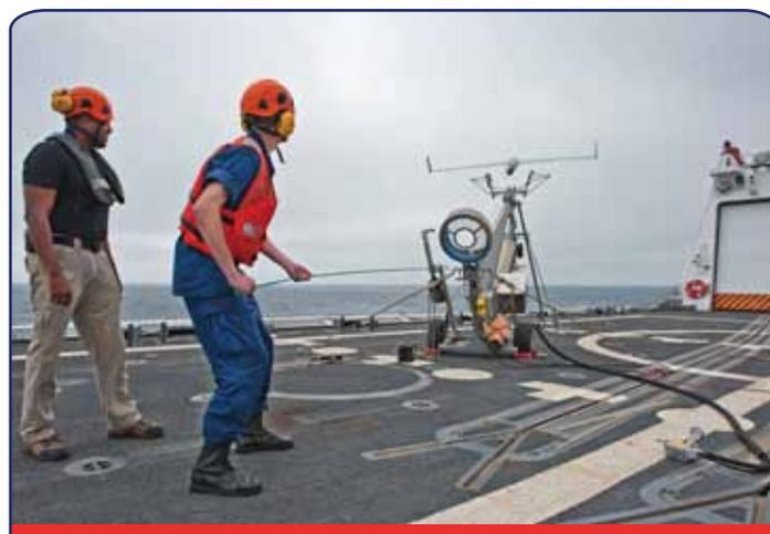
A Coast Guard Stratton crewmember launches a ScanEagle UAS during a demonstration, Aug. 12, 2012. The Coast Guard Research and Development Center (RDC) has conducted several UAS demonstrations both from land and onboard the Coast Guard's National Security Cutters to support development of a small UAS for NSC acquisition project.
